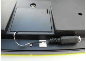
Now place the cable as you like and carefully close the battery compartment. Take care not to bend the cable - a small radius of down to approx. 1 mm is allowed.
