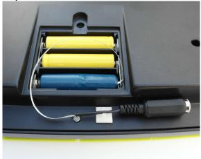
Insert the Power Supply Adapter (blue) into a suitable battery compartment and make sure that the polarity is correct:
