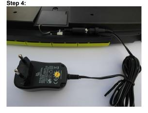
Finally connect the power supply to the socket on the Battery Supply Adapter. Take care not to overload the thin cable of the Battery Supply Adapter later on.
